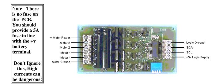
The Motor Ground and the Logic Ground are internally connected on the Module. Be sure to use cable rated for at least 5A for the Battery, Fuse and Motor leads.
